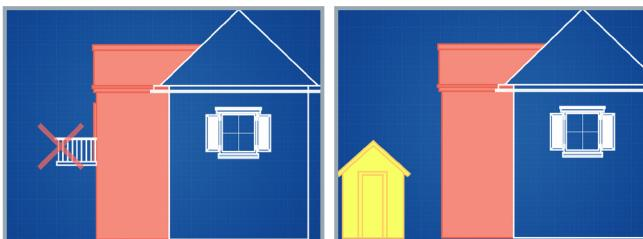
7. Any upper-floor window in a wall or roof slope in a side elevation must be obscure-glazed and non-opening unless the parts which can be opened are more than 1.7 metres above the floor of the room in which it is installed.
