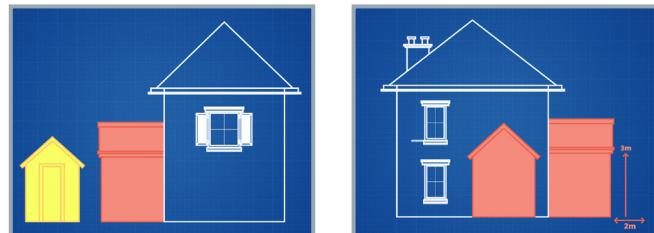
8. If extension is within two metres of a boundary maximum eaves height should be no higher than three metres to be permitted development.
